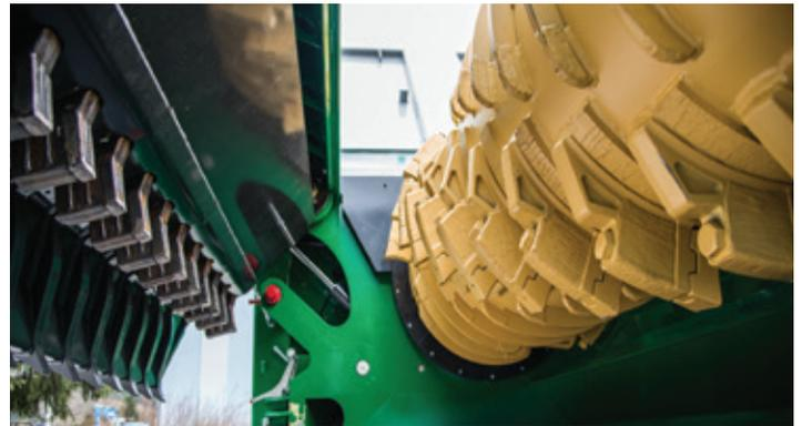
The Terminator is a low-speed, high-torque, single-shaft industrial shredder designed to process nearly all difficult waste types, including heavy C&D debris, bulky waste, white goods, mattresses, tires and municipal solid waste (MSW). Achieve a variety of output particle sizes with the adjustable cutting gap and counter comb. Easily swap shredding units to configure from coarse pre-shredding to defined shredding.
